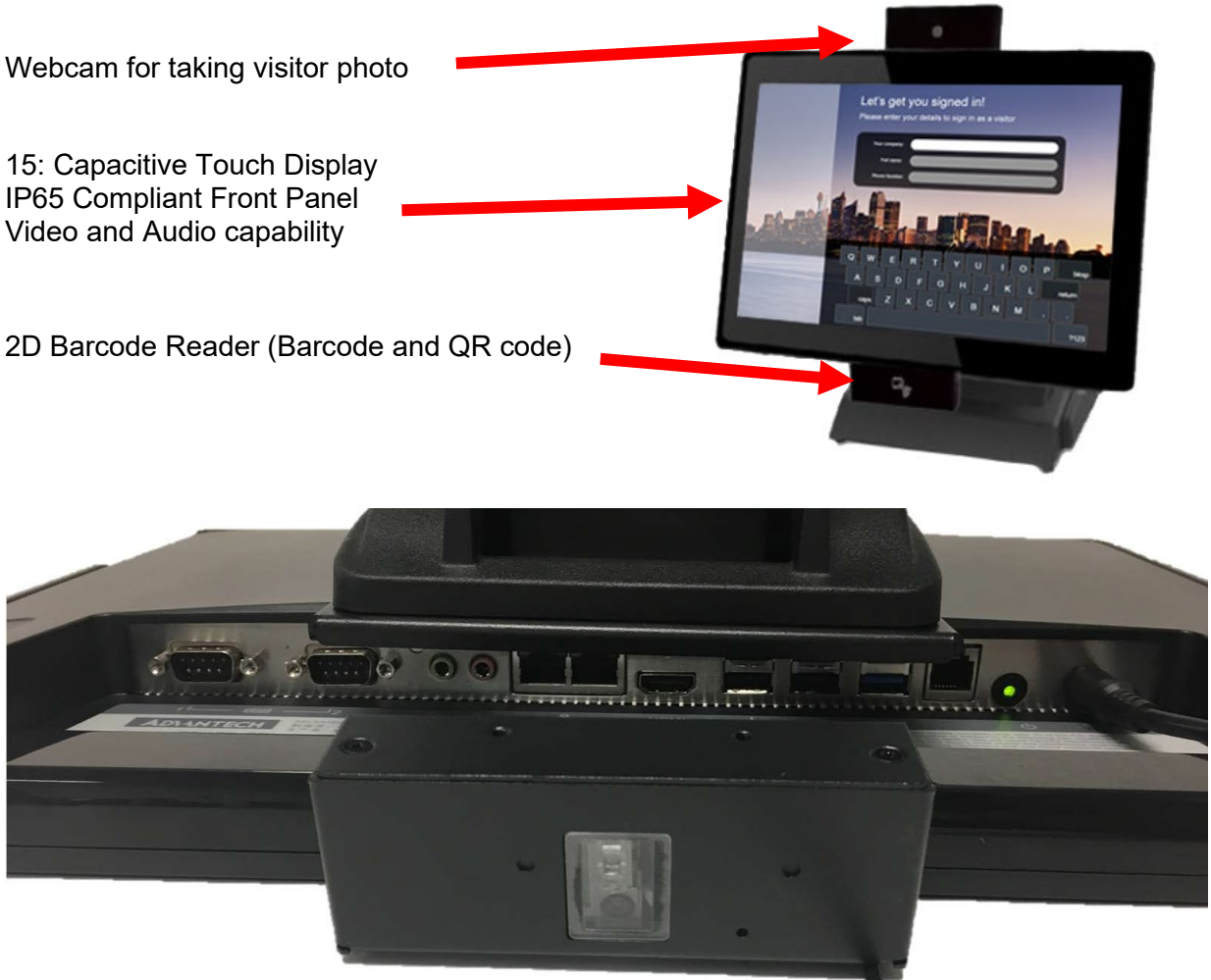
Underside of Desktop Kiosk showing inputs and options
