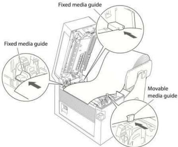
Align the label roll with the left fixed media guides (2 places), and align the right movable media guide with the media width.
